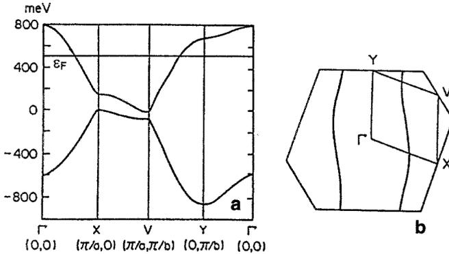
**Fig. 2.3.** (a) Calculated band structure and (b) Fermi surface of  $(\text{TMTSF})_2\text{AsF}_6$  representative for all  $(\text{TMTSF})_2X$ . From [43]
