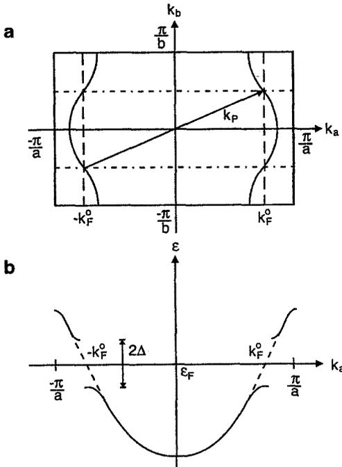
**Fig. 2.4.** (a) Schematic representation of a quasi 1D Fermi surface with nesting vector  $\mathbf{k}_P = (2k_F, \pi/b, 0)$ . The dash-dotted line is the resulting new Brillouin zone. (b) Opening of the Peierls gap  $2\Delta$  at  $\pm k_F$  in the dispersion relation
