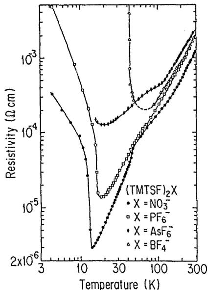
**Fig. 2.5.** Temperature dependence of the dc resistivity for various  $(\text{TMTSF})_2\text{X}$  salts in double-logarithmic scale. From [35]
