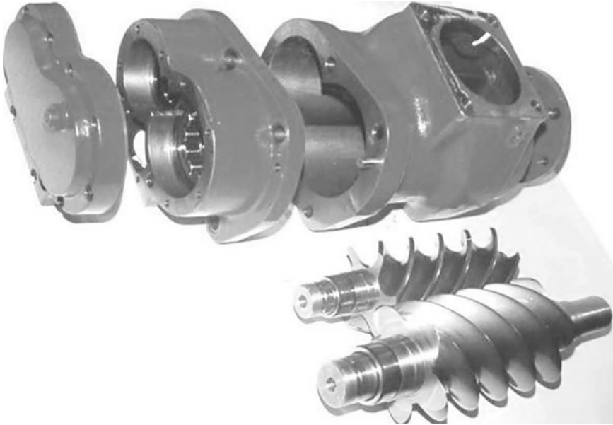
Fig. 1.4. Screw compressor mechanical parts
